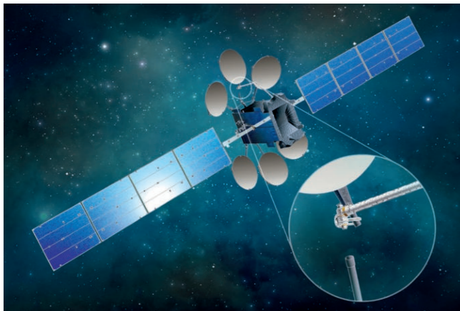
Photo on top: In this artist's rendering, the Dragonfly technology enables satellite self- assembly in orbit.
